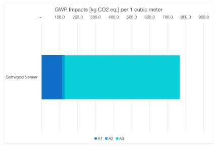
At a more granular level, we find lumber used accounts for 88% of combined A1 and A2 impacts. The emissions sources contributing the most within the manufacturing stage (A3) are natural gas and electricity, accounting for 55% and 26% of overall emissions, respectively.
