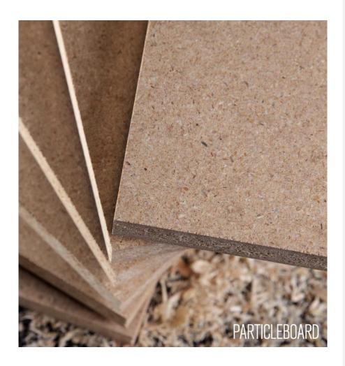
Timber Products manufactures both fir and pine particleboard substrates. Particleboard can be produced in all grades to fit your needs, including underlayment, door core, commercial, industrial, and specialty. Timber Products maintains certifications with Forest Stewardship Council (FSC) and SCS Global Services (for recycled content and no added formaldehyde).
